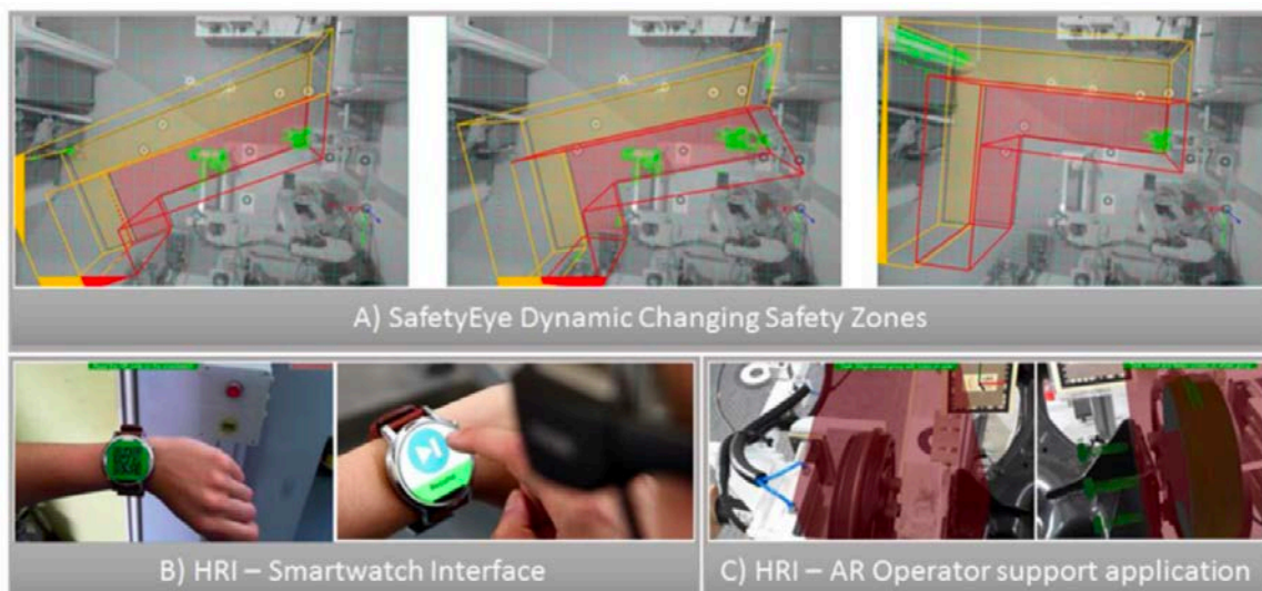
Figure 14 - Safety measures for human-robot collaboration assembly (Michalos et al., 2018)
